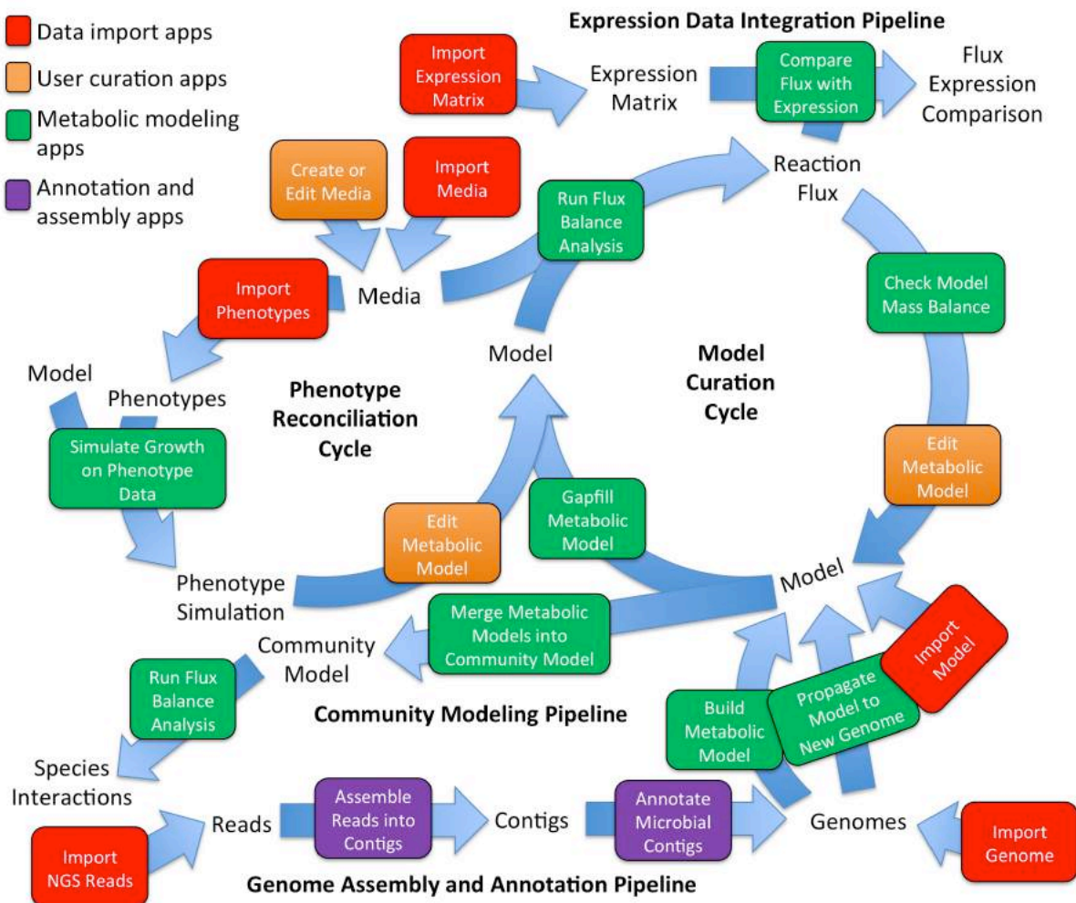
Figure 2. Workflows in KBase for assembly and annotation of genomes and reconstruction and analysis of metabolic models.
